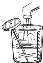
3. Check the temperature on the thermometer as the water is running into the cup.
